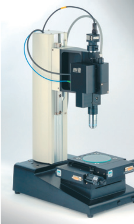
▲ Nano vibration analyzer for vibrational measurement of micro structures
